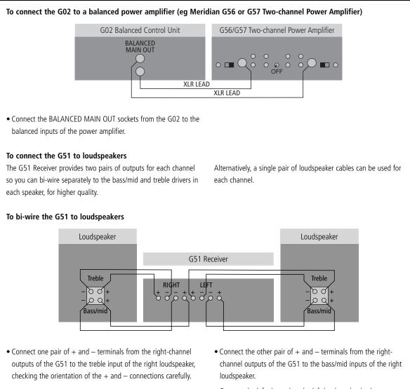
• Connect the left channel to the left loudspeaker in the same way.
