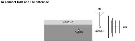
The DAB/FM tuner uses a single antenna input for both DAB and FM reception. For optimum reception we recommend using both DAB and FM antennae with an appropriate combiner.
