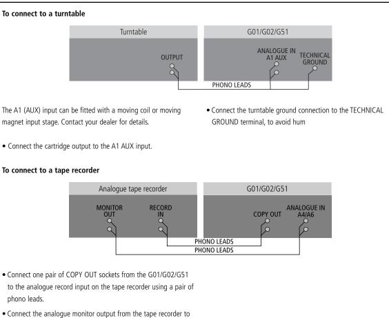
the A4 TAPE input on the G01/G51 or input A6 on the G02 using a pair of phono leads.
